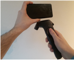
Figure 1: Phone player uses a phone in one of their hands and a controller to track their position in the other (no need for any holder as we wanted this to be as accessible as possible)
